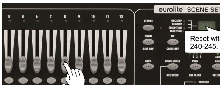
Set channel fader 8 to a value between 240 and 245 and reset the winch. In case of any malfunction, check the DMX connection.
