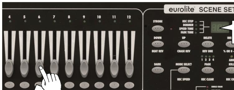
To test the DMX connection, pull up the channel fader 6 and observe the Space Ball's movement, then move the fader back down to 0.
