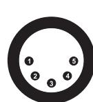
If you are using controllers with this occupation, you can connect the DMX-output of the controller directly with the DMX-input of the first fixture in the DMX-chain. If you wish to connect DMX-controllers with other XLR-outputs, you need to use adapter-cables.
