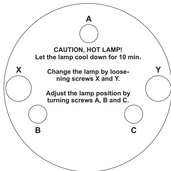
The lampholder is aligned at the factory. Due to differences between lamps, fine adjustment may improve light performance.
