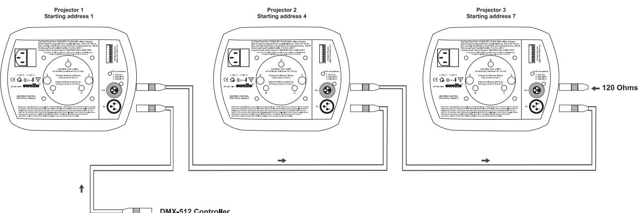
**! The wires must not come into contact with each other, otherwise the fixtures will not work at all, or will not work properly.**
